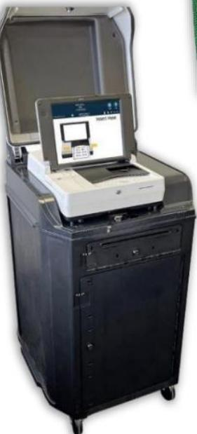
The **DS300 Ballot Scanner** (*New! formerly the DS200 scanner*) scans and tabulates all ballots and stores all the images on two thumb drives. A **Red** seal covers the thumb drive compartment but is changed to a **Blue** seal if the paper roll needs replacing, printer paper jams and needs to be reset, or if entire the Scanner box is replaced.
